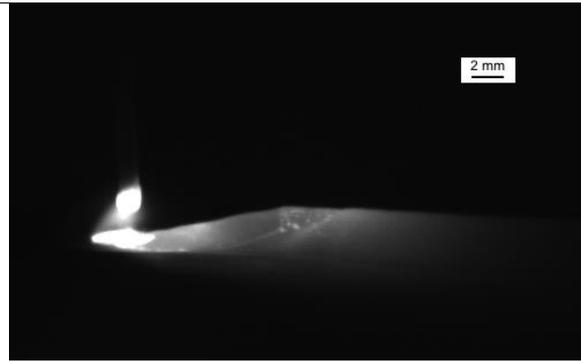
Figure 6: the weld pool length was evaluated to 15 mm from a snapshot of the deposition process.
