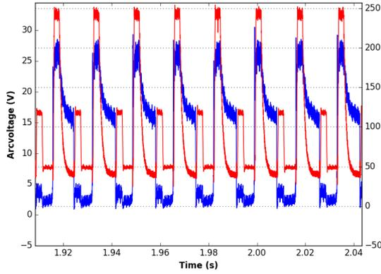
Figure 1: CMT electrical waveforms monitored during a deposition procedure (Arc Voltage is in blue and current is in red).
