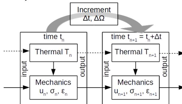
Figure 3: procedure of the thermo-mechanical simulation. First the thermal problem is solved at time  $t_n$  then the thermal loading is applied on the mechanical problem. At time  $t_{n+1}$ , the deposit geometry is updated by an addition of material and the thermal and mechanical problems are initialized with the previous computed data at  $t_n$ . The two computations are restarted for time  $t_{n+1}$ .
