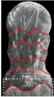
Figure 5: macrograph of the 5 deposits. The dashed line represents the initial shape of the substrate before the deposition of the 1<sup>st</sup> layer.
