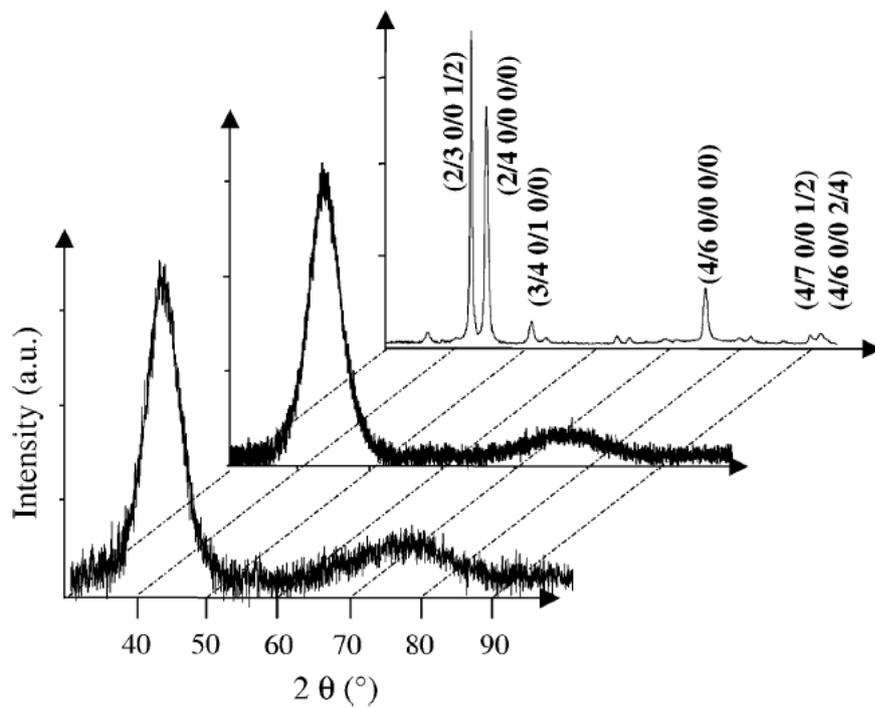
Figure 1 : X-ray diffraction patterns of the films prepared at a/ 298 K, b/ 373 K, and c/ 533 K. a.u. stands for arbitrary units.
