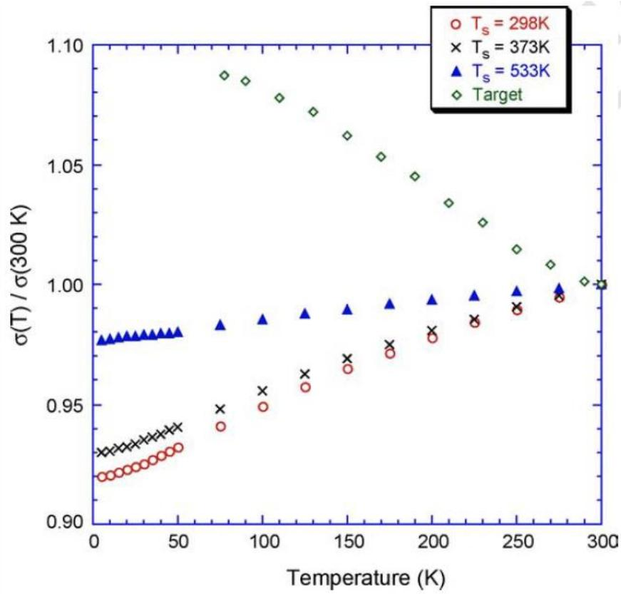
Figure 2: Temperature dependence of the normalized conductivity  $\sigma/\sigma(300 \text{ K})$  for the i- $\text{Ti}_{41.5}\text{Ni}_{17}\text{Zr}_{41.5}$  films and the  $\text{Ti}_{45}\text{Zr}_{38}\text{Ni}_{17}$  target.
