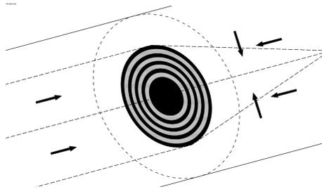
Figure 3: Individual Telescope, centred within opposing beams.
