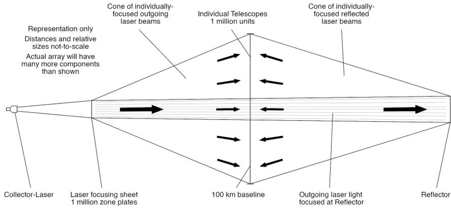
Figure 10: The Planet Seeker Interferometer, side view, showing the position-keeping lasers.
