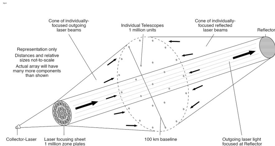
Figure 1: The Planet Seeker Interferometer, in a three-quarters orthographic projection, showing the position-keeping lasers.
