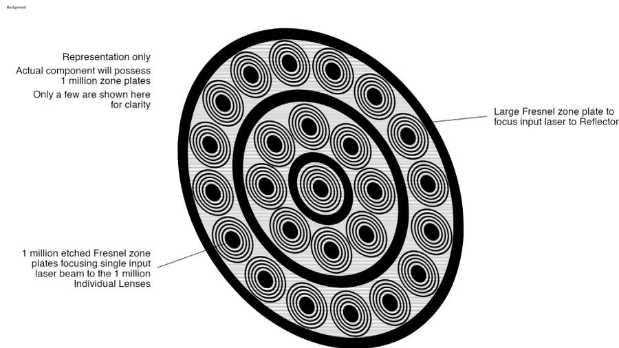
Figure 5: Laser focusing sheet, shown in a three-quarters orthographic projection.
