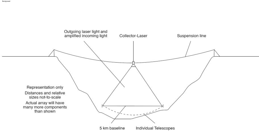
Figure 9: Ground-based prototype of the Planet Seeker Interferometer, shown situated in a hypothetical mountain valley.
