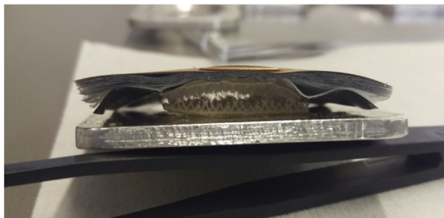
Fig. 19. MLI side view. It can be seen the strong degradation of the velcro.
