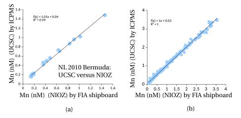
Figure 2. The correlation between the two methods of analysis for the determination of  $[Mn_{diss}]$  at GA02 (shipboard and laboratory mass spectrometry): (a) at Bermuda; (b) all 55 west Atlantic stations.
