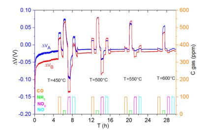
$\label{eq:sensors} Figure \ 1: Responses \ of \ Au-15\% V_2O_5 \ electrode \ YSZ \ based \ sensors \ to \ CO, \ NH_3, \ NO_2 \ and \ NO \ at \ temperatures \ of \ 450, \ 500, \ 550 \ and \ 600^\circ C.$
