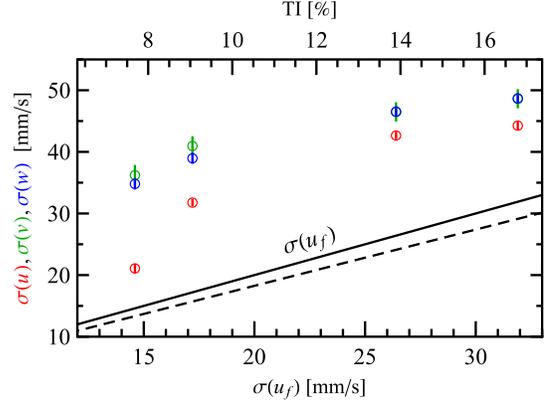
FIG. 3. Standard deviation of the bubble velocities ( $u, v, w$ ) vs the standard deviation of the flow velocity. The bubble velocity fluctuations exceed that of the fluid (solid line). The dashed line  $\sigma(u_{\mu b})$  is for microbubbles at  $Re_\lambda = 62$  [49], obtained from fitting their data,  $\sigma(u_{\mu b}) \approx 0.9\sigma(u_f)$ .
