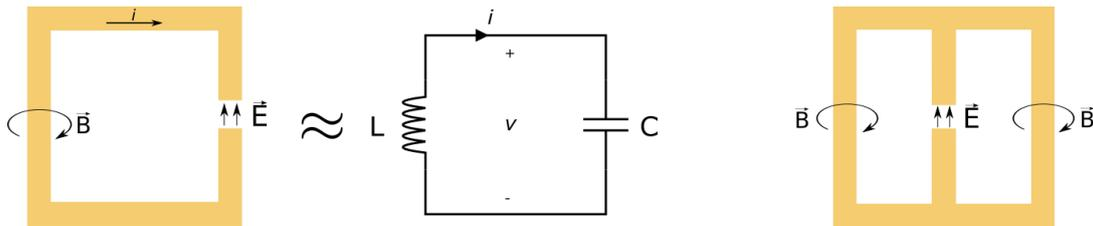
Figure 4: Left: simplest example of SRR with its equivalent circuit, the resonance frequency is given by  $\omega_0 = 1/\sqrt{LC}$ . Right: the design we have chosen for our study, the magnetic field inside each loop is oriented in opposite direction.
