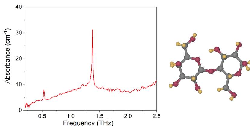
Figure 2: Left - spectrum of a powder of  $\alpha$ -Lactose monohydrate. The sample volume is  $\sim 15$  nL corresponding to a mass of  $\sim 23$   $\mu$ g. Right - schematic view of the lactose molecule.
