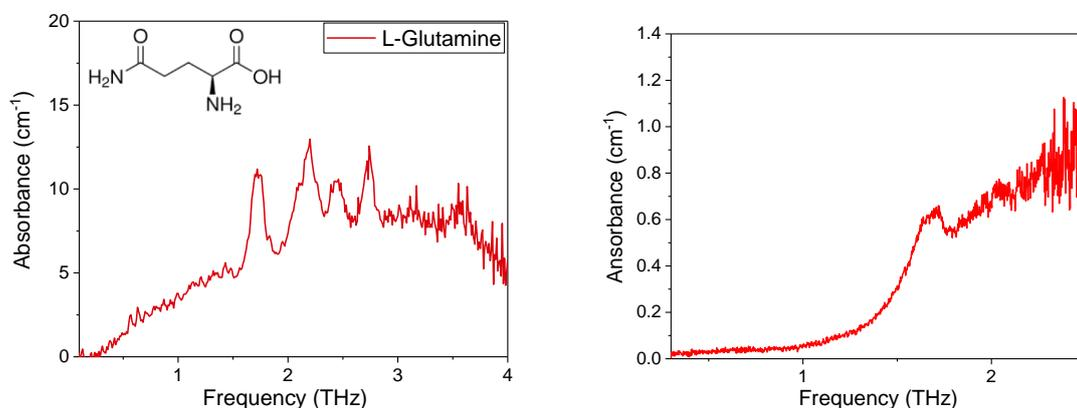
Figure 3: Spectrum of glutamine [ $C_5H_{10}N_2O_3$ ] samples. Left - 6.8  $\mu$ g of powder (volume of about 5 nL), right - 250 ng of dried solution (volume of dried solution of about 200 pL). We cut the spectrum at 2.5 THz for the dried solution because of the lower signal-to-noise ratio.
