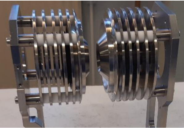
Figure 16. Picture of MORATrap on its mechanical support. It has been machined and assembled at LPC Caen.
