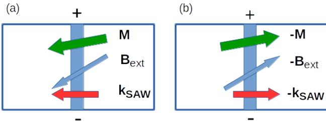
FIG. 3. Sketch of the sample (substrate and bilayer). (a) and (b) display two configurations of in-plane external magnetic field  $\mathbf{B}_{\text{ext}}$ , magnetization  $\mathbf{M}$  and  $\mathbf{k}_{\text{SAW}}$ . (b) is obtained from (a) by inversion of  $\mathbf{B}_{\text{ext}}$ ,  $\mathbf{M}$  and  $\mathbf{k}_{\text{SAW}}$ . The voltage is measured between the (+) and (-) terminals.
