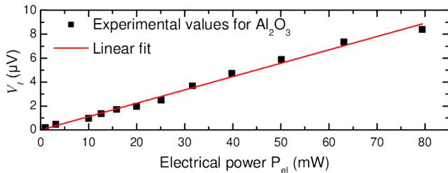
FIG. 2.  $V_I$  (proportional to the spin current amplitude) as function of incident electrical power on IDT for  $\text{Al}_2\text{O}_3/\text{Co}/\text{Pt}$  sample. The red line is a linear fit, in good agreement, with the data<sup>23</sup>.
