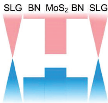
Fig. 31 SLG/h-BN/MoS 2 /h-BN/SLG structure: blue is the valence band and pink is the conduction band. Adapted from ref. 106.
