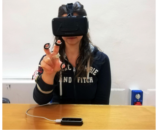
Fig. 1: Haptic hand guidance using vibrations in a demonstrative Virtual Reality scenario. The user wears the haptic thimbles and orients the hand following the cues displayed at the user’s finger pulps. The fingertips and the palm positions are tracked by a Leap Motion device placed on the table.
