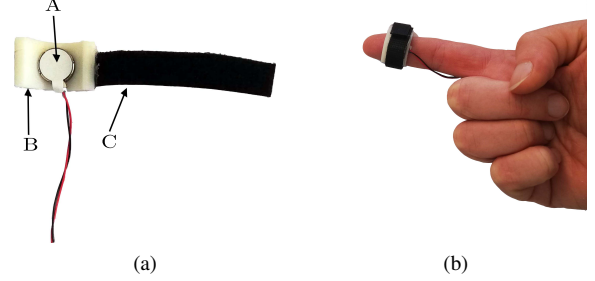
Fig. 3: The vibrotactile cutaneous thimble. A vibromotor (A) is enclosed on a 3D printed thimble (B). A Velcro® belt (C) enables the user to easily fasten the device on the finger. The total weight of the thimble is 3.02 g.
