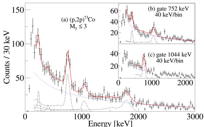
FIG. 5. (Color online) (a) Doppler-corrected  $\gamma$ -ray spectrum for  $^{73}\text{Co}$  populated via the  $(p, 2p)$  reaction.  $\gamma$ - $\gamma$  coincidence spectra are shown as insets without background subtraction and all  $M_\gamma$ , a gate on 752-keV, (b), and a gate on 1044-keV (c). Individual response functions for each transition are shown as long-dashed black curves, background as short-dashed red curves, and data fits as solid red curves.
