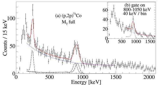
FIG. 4. (Color online) (a) Doppler-corrected  $\gamma$ -ray spectrum for  $^{71}\text{Co}$  populated via the ( $p, 2p$ ) reaction. Inset (b) shows the  $\gamma$ - $\gamma$  coincidence spectrum with a gate on the 800 – 1050 keV region and considering all  $M_\gamma$  (background is not subtracted). Individual response functions for each transition are shown as long-dashed black curves, background as short-dashed red curves, and data fits as solid red curves.
