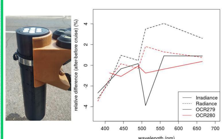
Fig 7: Sensors were calibrated before and after lovapm006d deployment. Sensor drift after 2 months in the med sea stays reasonable. Pictures of the sensor just after the recovery and without any cleaning.
