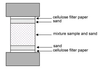
Fig. 3. Packing of ASE extraction cell
