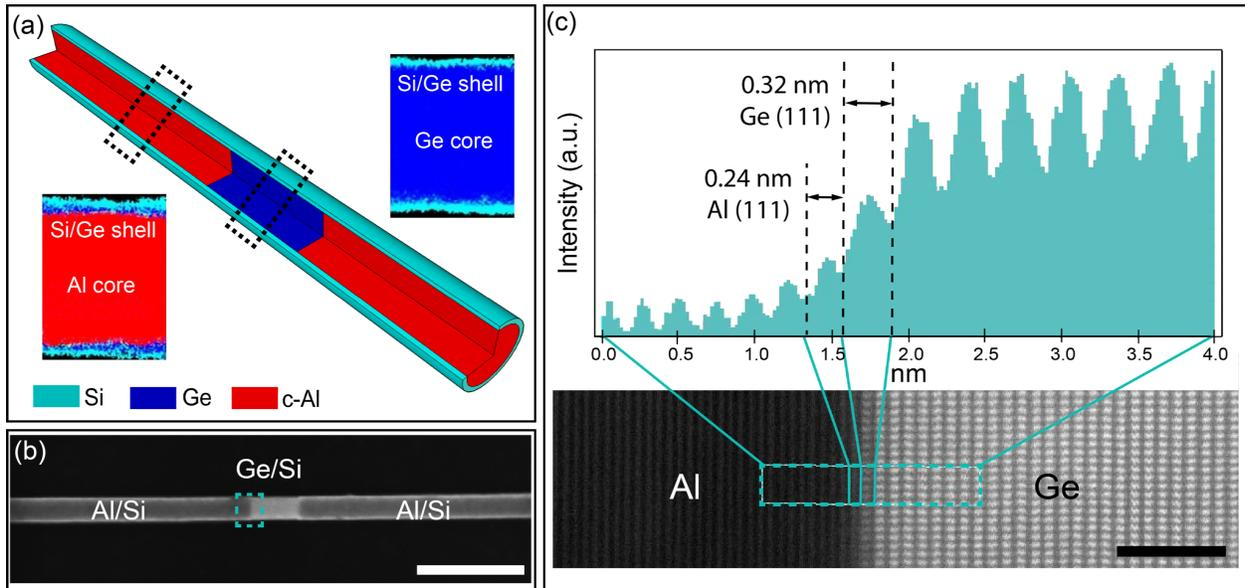
**Figure 1.** (a) Schematic illustration of an axial Al-Ge-Al NW heterostructure with an ultra-thin semiconducting shell wrapped around. The insets show EDX chemical maps at the respective positions along the heterostructure indicating an intact semiconducting shell around the entire Al-Ge-Al heterostructure. (b) SEM image of the actual heterostructure arrangement. Scale bar is 200
