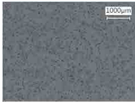
(b) Pores within an adhesive joint after 12h at ambient temperature
