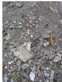
Demolition rubble (0-40 mm)
