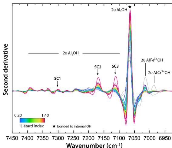
**Fig 2.** Secondary derivative spectra of the 7000  $\text{cm}^{-1}$  doublet (1.4  $\mu\text{m}$ ) of terrestrial kaolinite samples. Spectra are colored according to the Liétard Index values that increase with the degree of crystalline order. Grey spectra indicate kaolinite samples that were not analyzed through XRD measurements. Black arrows indicate spectral contributions that shift according to the crystallinity of the samples.
