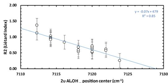
**Fig 3.** Diagram illustrating the relationship between the crystallinity of kaolinite and its near-infrared signature as seen through the representation of the Liétard Index values as a function of the position shift of the 7120  $\text{cm}^{-1}$  peak position.
