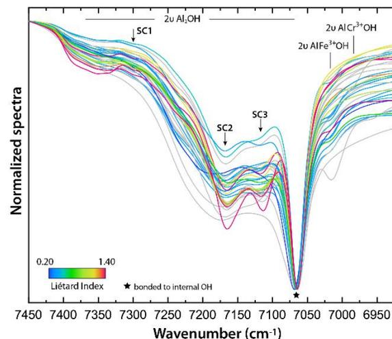
**Fig 1.** Reflectance spectra of the  $7000\text{ cm}^{-1}$  doublet ( $1.4\ \mu\text{m}$ ) of terrestrial kaolinite samples. Spectra are colorized according to the Liétard Index values that increase with the crystallinity order. Grey spectra are for kaolinite samples that were not analyzed through XRD measurements. Black arrows indicate spectral contributions that shift according to the crystallinity of the samples.
