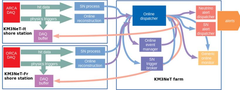
Figure 3: Functional diagram of the KM3NeT DAQ system and online framework outlining the information exchange between the two shore stations and the central farm dedicated to the real-time processing applications.
