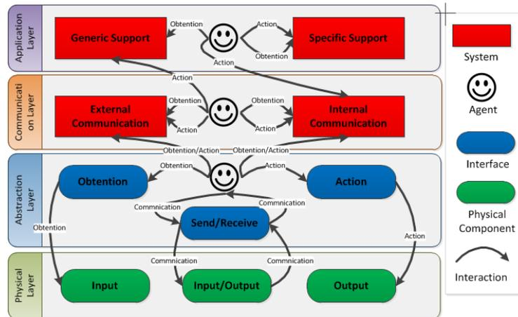
Fig. 2. Multi-layered architecture for an IoT application
