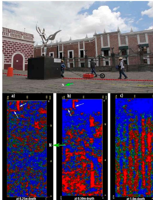
**Fig. 8.** Photo of S3 area in the front of “Aguadores” prospected with the 200 MHz antenna. a), b) and c) below show three depth slices at 25 cm, 50 cm and 1.5 m depth respectively. The structure indicated by the white arrows could probably correspond to an ossuary.
