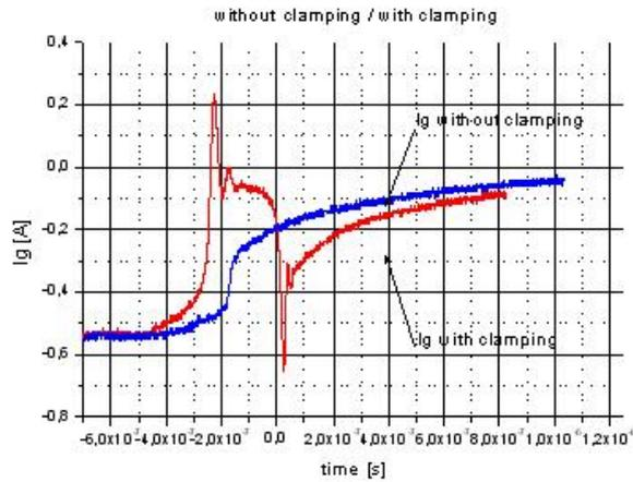
Fig. 1.  $I_g$  with and without clamping
