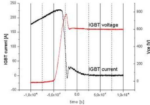
Fig. 8. Turn off of the IGBT, 230A, 600V
