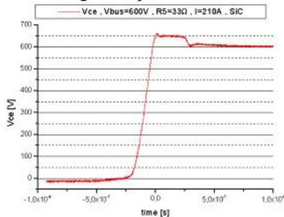
Fig. 9. Clamping with SiC diode ( $D_2$ )
