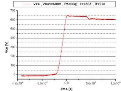
Fig. 10. Clamping with BY228 diode ( $D_2$ )
