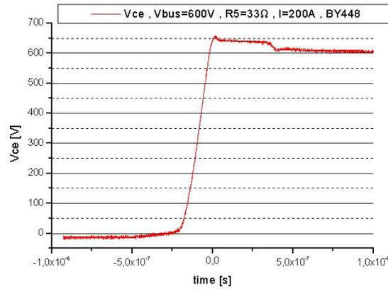
Fig. 11. Clamping with BY448 diode ( $D_2$ )
