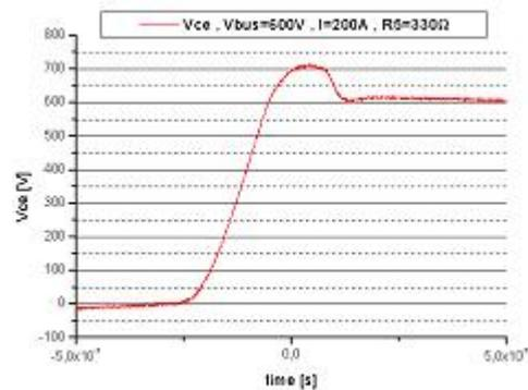
Fig. 13. Clamping with  $R_5=330\Omega$
