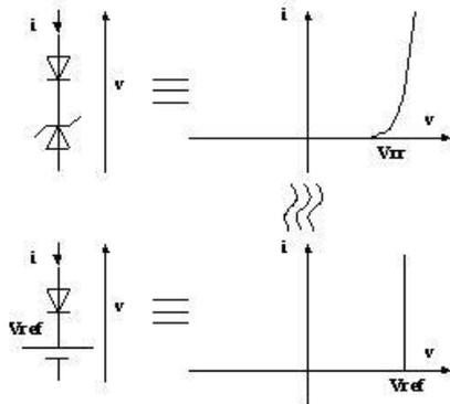
Fig. 4. Equivalence between transil diode and voltage source
