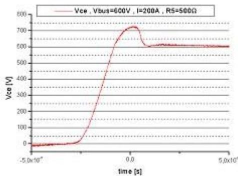
Fig. 12. Clamping with  $R_5=500\Omega$
