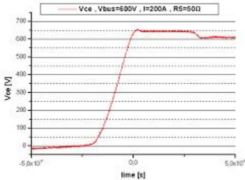
Fig. 16. Clamping with  $R_5=50\Omega$
