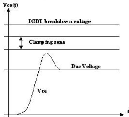
Fig. 2.  $V_{ce}$  during the turn off of IGBT (normal operation)
