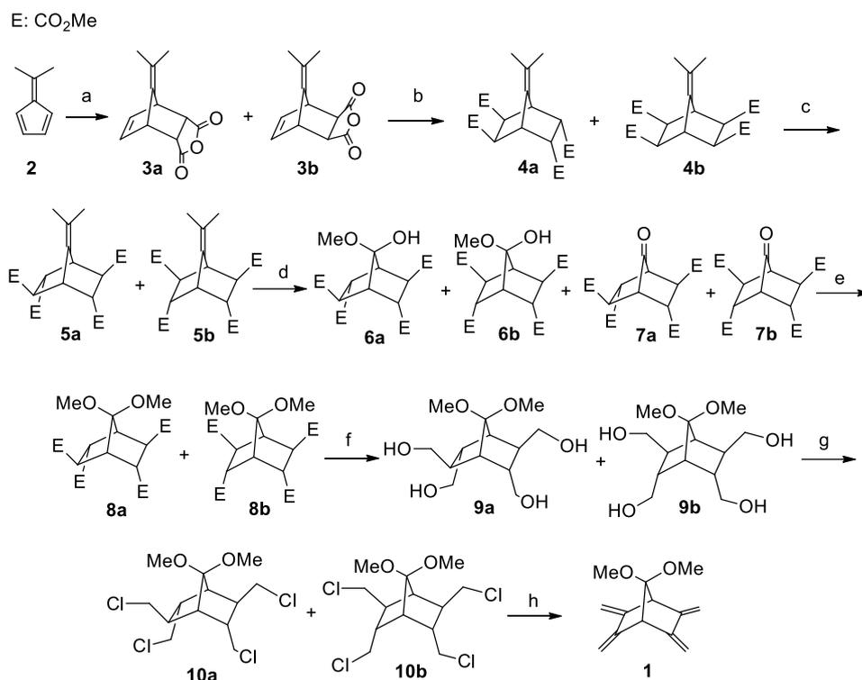
**Scheme 2.** Synthesis of **1**. a) maleic anhydride, DCM; 86% b) Pd/C, CuCl<sub>2</sub>, CO, MeOH; 74% c) K<sub>2</sub>CO<sub>3</sub>, MeOH; 88% d) O<sub>3</sub>, Me<sub>2</sub>S, DCM-MeOH; e) HC(OMe)<sub>3</sub>, APTS, MeOH; 82% for two steps f) LiAlH<sub>4</sub>, THF; 94% g) Cl<sub>2</sub>, PPh<sub>3</sub>, imidazole, DCM-ACN-pyridine; 68% h) *t*-BuOK, DMF; 61%.
