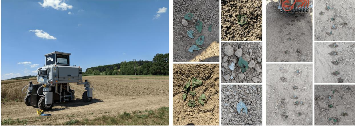
Figure 14: Left: example picture of field robot performing weed control evaluation. Middle: sample pictures of leaves after mechanical weed removal. Right: sample pictures after selective spraying.
