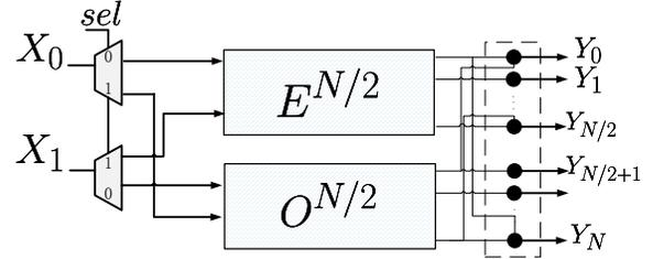
**Fig. 2.** General structure of the order-64 inverse DCT-II. Blocks  $O^{N/2}$  corresponds to odd decomposition and  $E^{N/2}$  to the even decomposition of  $[C_2^N]^T$ .  $X_0$  and  $X_1$  denote the input samples, while  $Y_i$  denote the outputs.
