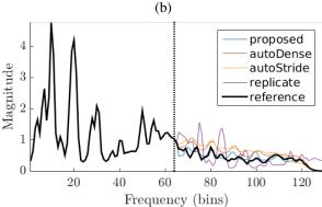
**Fig. 2**. Examples of predictions for (a) the *medley-solos-db* dataset and (b) the *gtzan* dataset. The proposed model handles correctly the harmonic structures (a) and the average magnitude of more complex spectral shapes (b).
