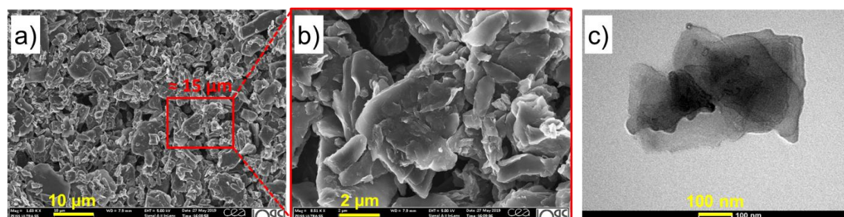
Figure S1: a) and b) SEM micrographs of the GDL/GA (0.4 mg cm -2 ) porous network at different magnifications c) TEM micrograph of a GA sheet
