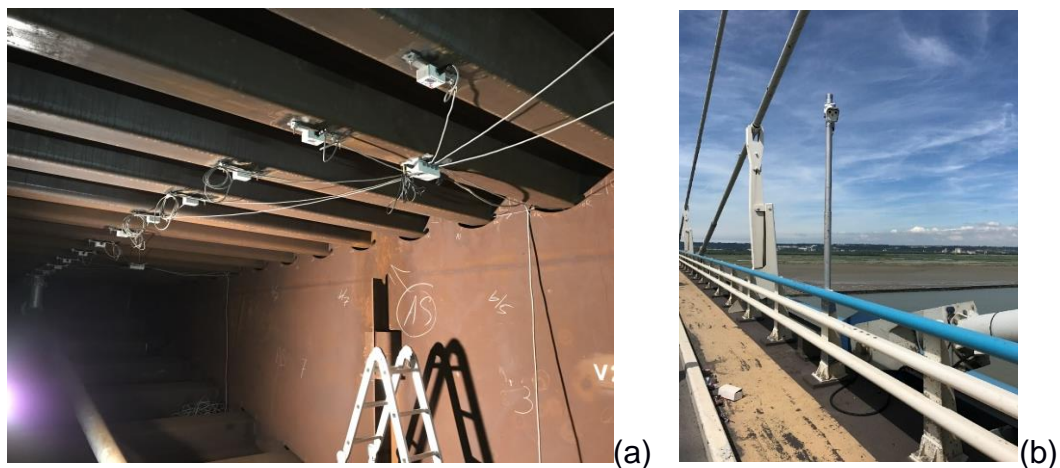
Figure 6 – SiWIM in the Normandy bridge: (a) extensometers under the longitudinal stiffeners in the box, (b) camera on the bridge deck
