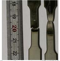
Figure 4: Two tensile test specimen of TA6V/21S after break
