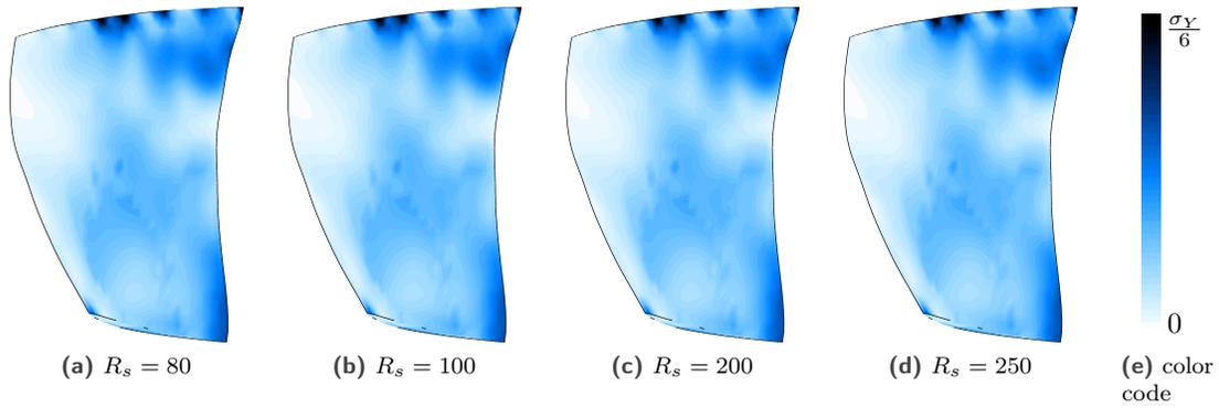
Figure 8. Blade stress fields for different  $R_s$  values.
