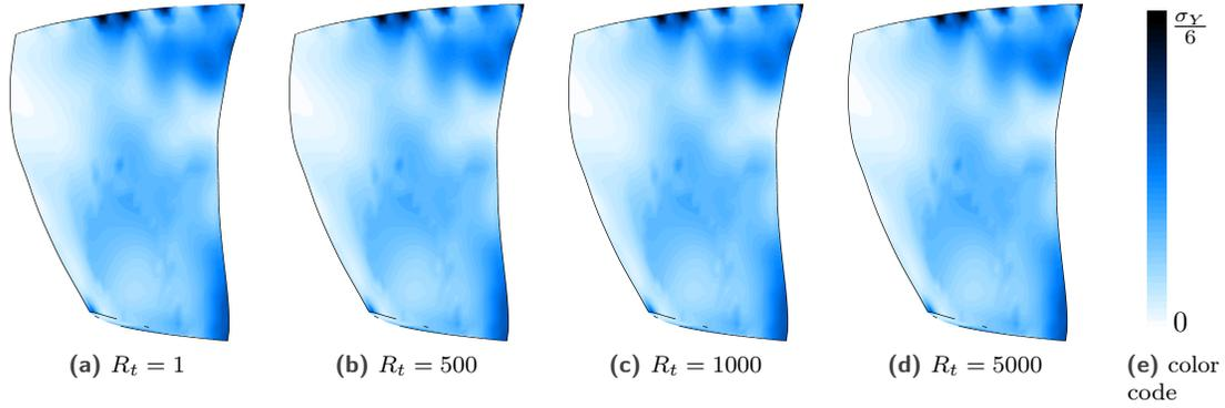
Figure 9. Blade stress fields for different  $R_t$  values.
