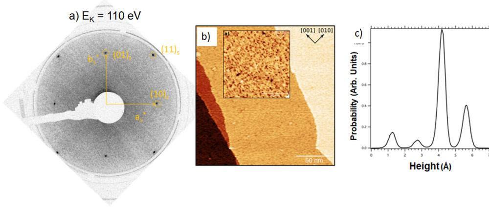
Figure 6: Structure of the  $\text{Fe}_{0.85}\text{Al}_{0.15}(100)$  surface: (a)  $(1 \times 1)$  LEED patterns after annealing at 973 K. Spot indexes are shown; (b) STM image after annealing at 1078 K ( $200 \times 200 \text{ nm}^2$ ,  $U_b = 0.9 \text{ V}$ ,  $I_t = 0.1 \text{ nA}$ ) with a zoom in insert ( $50 \times 50 \text{ nm}^2$ ,  $U_b = 1.6 \text{ V}$ ,  $I_t = 0.4 \text{ nA}$ ); (c) Corresponding histogram of the height of each pixel over the entire STM image.
