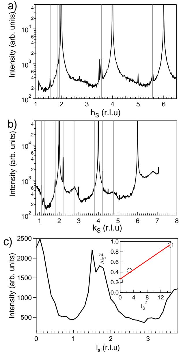
Figure 3: In plane radial diffraction scans ( $l = 0.075$ ) of a clean  $\text{Fe}_{0.85}\text{Al}_{0.15}(110)$  surface annealed at 1050 K (black line) along reciprocal directions a)  $(h_S, 0, 0.075)$ , b)  $(0, k_S, 0.075)$ . Grey lines point at peaks due to the surface reconstruction. c) Out-of-plane  $l_S$  scan on the reconstruction peak ( $h_S = 0, k_S = 2.2$ ). The inset shows the peak width analysis.
