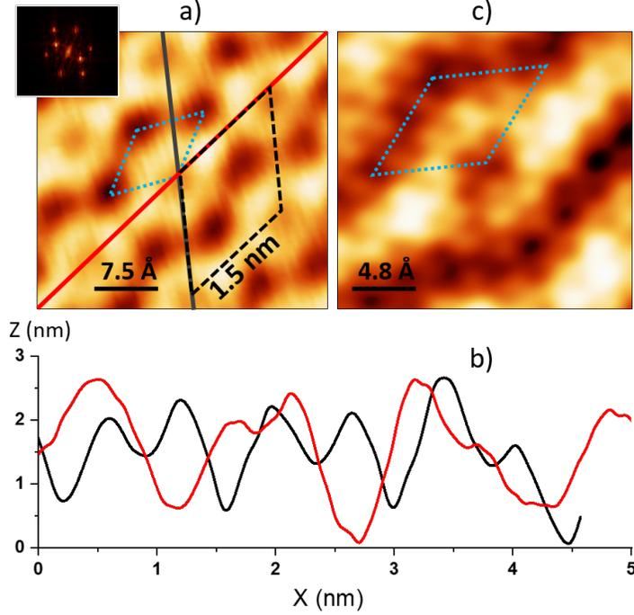
Figure 5: High resolution STM images ( $U_b = 2.5$  V,  $I_t = 0.05$  nA) of  $\text{Fe}_{0.85}\text{Al}_{0.15}(110)$  surface annealed at 1193 K a) ( $3.75 \times 3.75$ )  $\text{nm}^2$  and b) ( $2.4 \times 2.4$ )  $\text{nm}^2$ . Black and red lines in Fig. a are indicating profiles given in Fig. b. Black and blue rhombs highlight two periodic structures corresponding to reconstruction unit cell and areas with a lower density of states, respectively.
