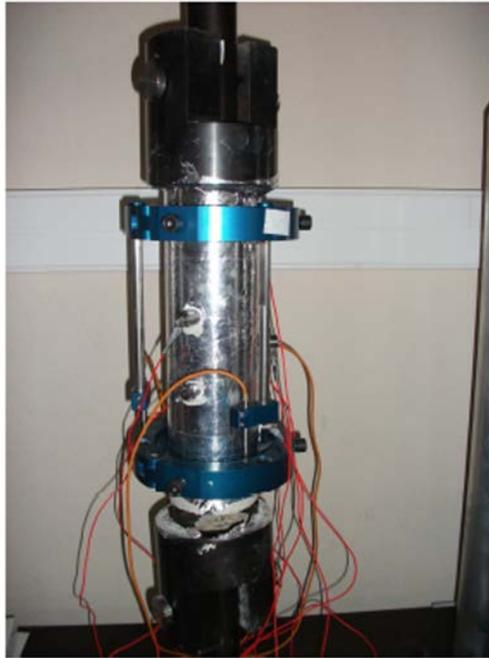
**Figure 7.10.** *Localization of the macro-crack in the concrete specimen under 85% traction creep*
