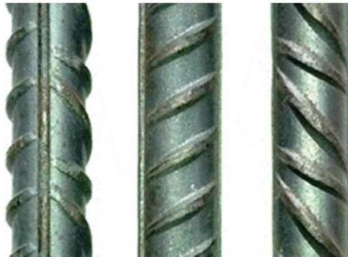
**Figure 6. High adhesion steel used.**
