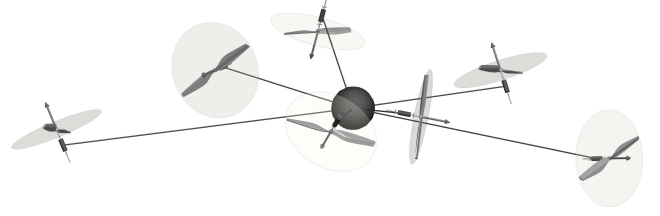
Figure 26. Conceptual 3D kinematic representation of the heptarotor design presented in (Nikou et al. (2015)).
