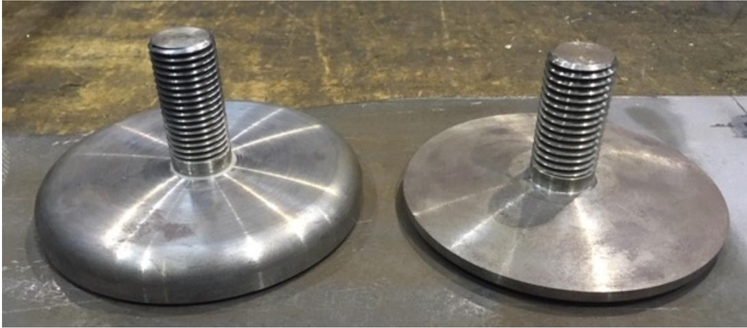
**Fig. 4:** Photo of studied C-Claw<sup>TM</sup> steel fastener T on the left and S on the right.
