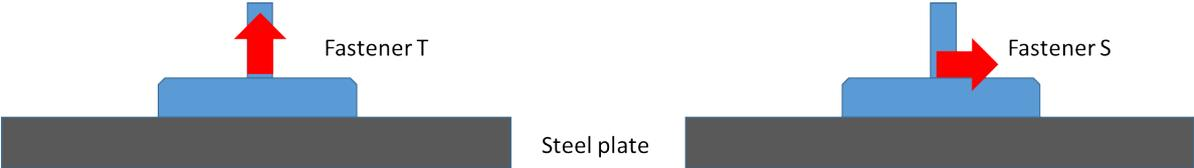
**Fig. 5:** Scheme of the two tested sollicitation modes: Tension and Shear loadings.
