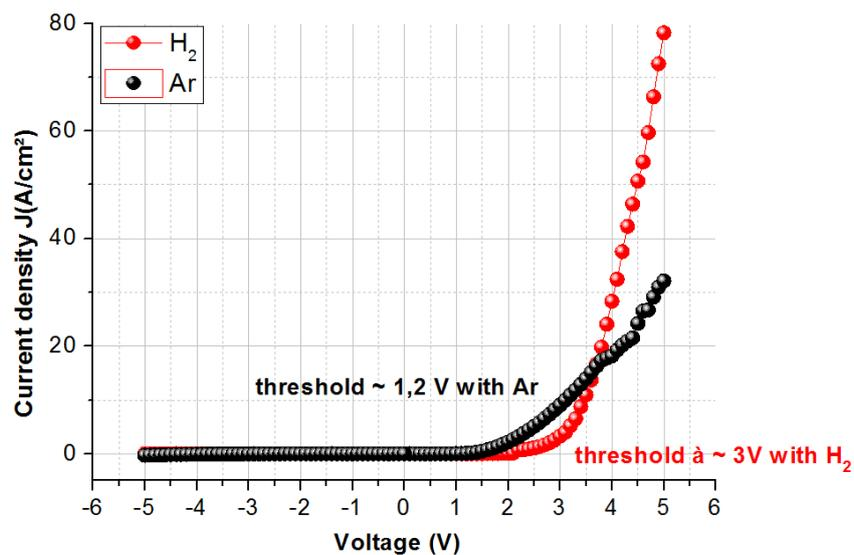
Figure 3 : Current-voltage characteristics in forward bias for P/N junctions in which  $P^+$  material was grown by VLS : Ar carrier gas (●) vs  $H_2$  carrier gas (●)
