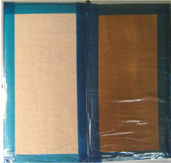
Figure 3: Preform with both reinforcements: untreated (left) and treated (right).
