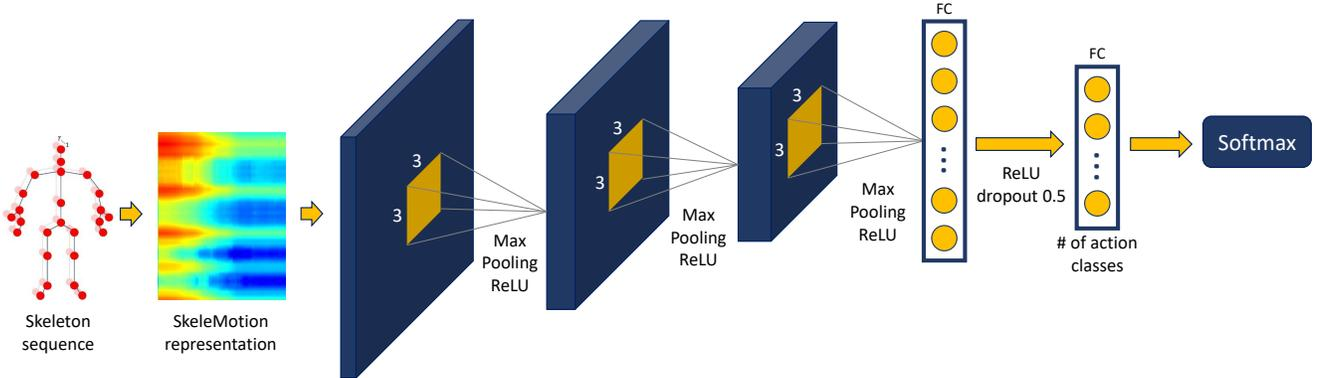
Figure 2. Network architecture employed for 3D action recognition.
