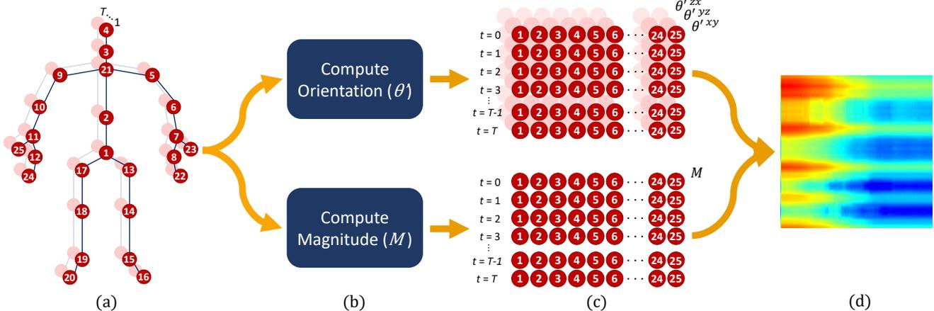
Figure 1. SkeleMotion representation. (a) Skeleton data sequence of  $T$  frames. (b) Computation of the magnitude and orientation from the joint movement. (c)  $\theta'$  and  $M$  arrays: each row encodes the spatial information (relation between joint movements) while each column describes the temporal information for each joint movement. (d) Skeleton image after resizing and stacking of each axes.
