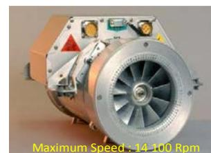
Fig.1. Picture of the whole fan from SAFRAN-Technofan
