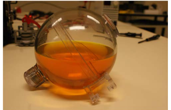
Fig. 5 Tank half filled with Novec liquid on earth
