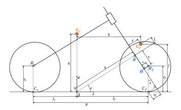
Figure 1: Sharp' two-body motorcycle kinematics
