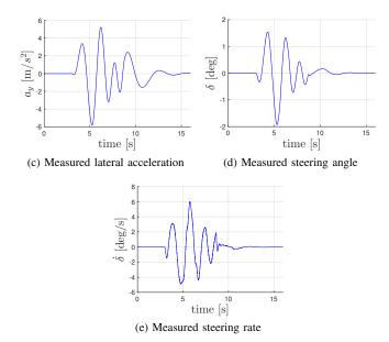
Figure 6: Measured states during the slalom
