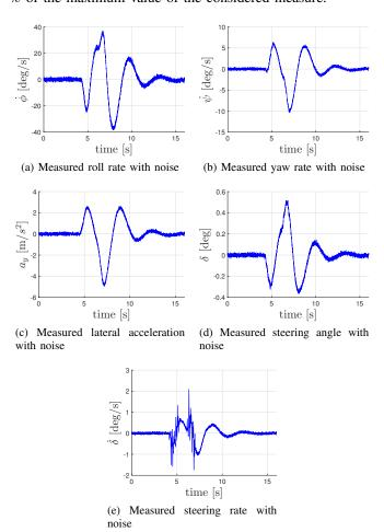
Figure 9: Measured states with noise during the DLC
