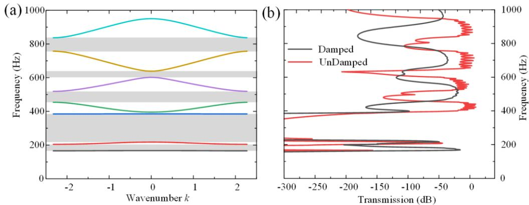
Figure 5 (a) Dispersion curves for the undamped infinite ABH shell and (b) Transmissibility for the finite 10 cells ABH shell.
