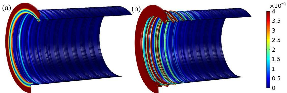
Figure 7 vibration shape at (a) 486 Hz (center of the third stop band), (b) 560 Hz (center of the third pass band).
