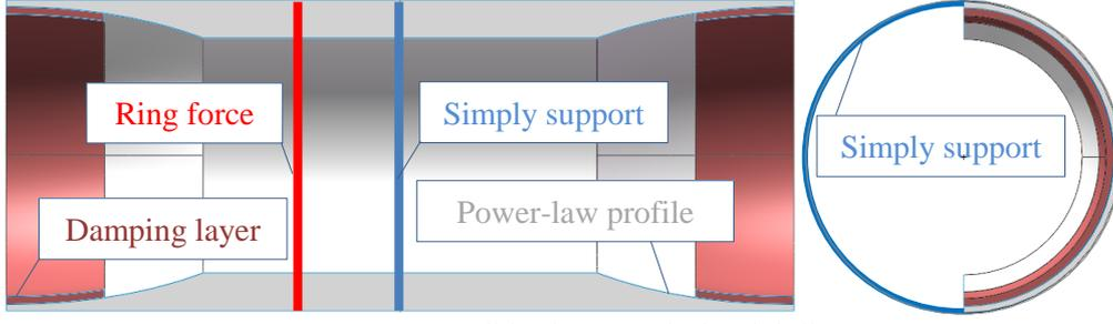
Figure 2 Unit cell for the ABH cylindrical shell.
