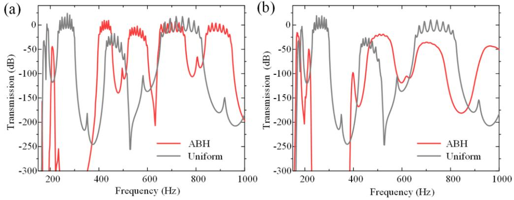
Figure 6 Comparison between the transmissibilities of the uniform and ABH cylindrical shells, (a) undamped shells, (b) damped shells.
