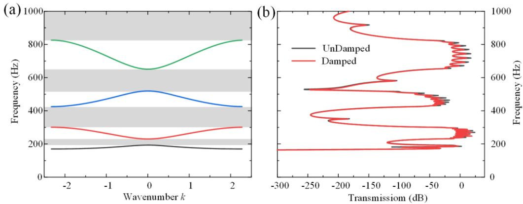
Figure 3 (a) Dispersion curves for the undamped infinite uniform shell (b) Transmissibility for the finite 10 cells uniform shell.
