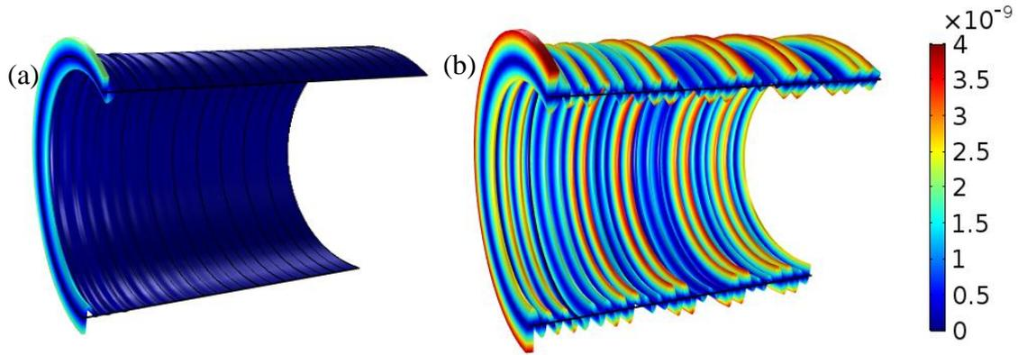
Figure 4 Vibration shape at (a) 585 Hz (center of the third stop band), (b) 738Hz (center of the third pass band)
