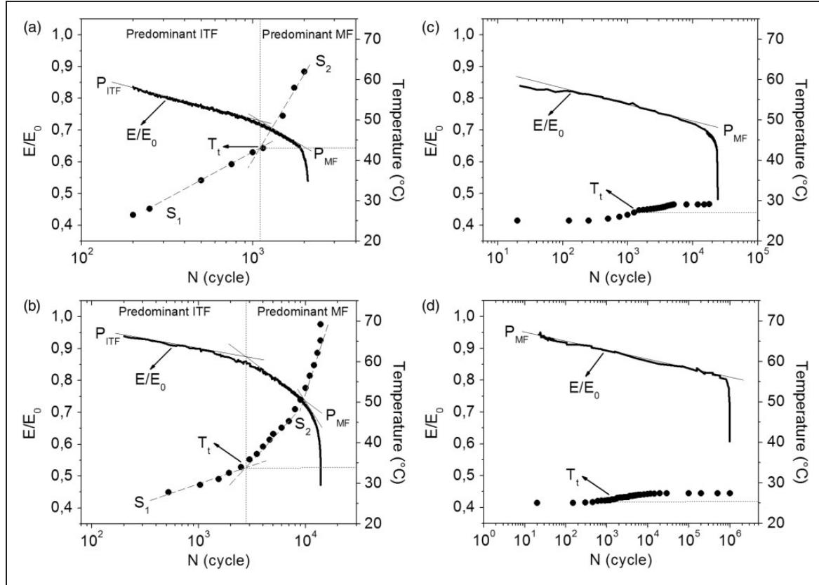
**Figure 11.** Evolutions of the relative Young's modulus ( $E/E_0$ ) and the self-heating phenomenon during fatigue tests: (a)  $f = 100$  Hz and  $\sigma_{\max} = 0.55 \sigma_{r(RO)}$ , (b)  $f = 100$  Hz and  $\sigma_{\max} = 0.40 \sigma_{r(RO)}$ , (c)  $f = 10$  Hz and  $\sigma_{\max} = 0.55 \sigma_{r(RO)}$  and (d)  $f = 10$  Hz and  $\sigma_{\max} = 0.40 \sigma_{r(RO)}$ .
