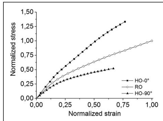
**Figure 4.** Normalized quasi-static tensile behavior of A-SMC composite at room temperature. One can mention that normalized stress (respectively strain) = stress (respectively strain)/ultimate stress (respectively strain) obtained for tests performed on RO-A-SMC serving as a reference.
