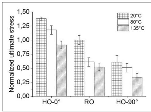
**Figure 5.** Normalized ultimate stress of oriented and nonoriented samples at 20°C, 80°C, and 135°C; (normalized value = current value/average ultimate stress ( $\sigma_r$ ) value obtained for tests performed at 20°C on RO-A-SMC).
