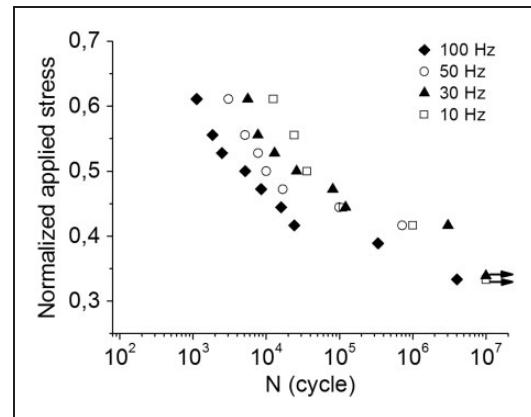
**Figure 9.** Normalized Wöhler curves at different frequencies for RO samples.
