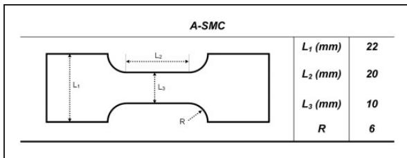
**Figure 2.** Optimized specimen geometry and its related dimensions.
