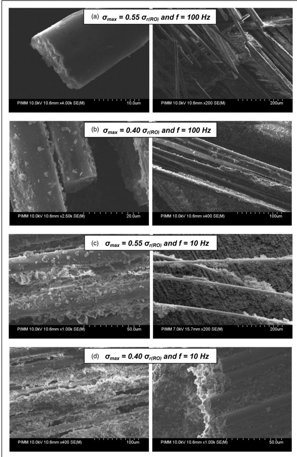
**Figure 13.** Fracture surface observation performed at different loading conditions: (a)  $\sigma_{max} = 0.55 \sigma_{r(RO)}$  and  $f = 100 \text{ Hz}$ , (b)  $\sigma_{max} = 0.40 \sigma_{r(RO)}$  and  $f = 100 \text{ Hz}$ , (c)  $\sigma_{max} = 0.55 \sigma_{r(RO)}$  and  $f = 10 \text{ Hz}$  and (d)  $\sigma_{max} = 0.40 \sigma_{r(RO)}$  and  $f = 10 \text{ Hz}$ .
