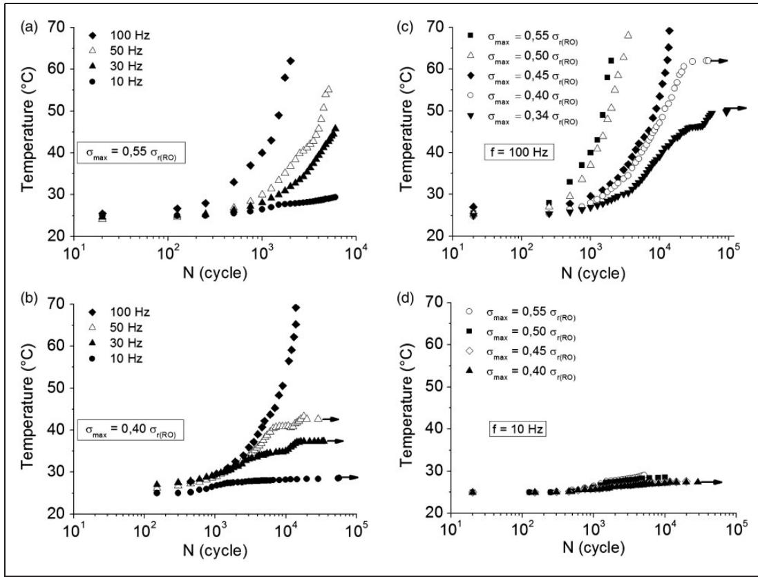
**Figure 10.** Temperature variation at different frequencies and amplitudes for RO samples: (a)  $\sigma_{\max} = 0.55 \sigma_{r(\text{RO})}$  and different frequencies, (b)  $\sigma_{\max} = 0.40 \sigma_{r(\text{RO})}$  ultimate stress and different frequencies, (c)  $f = 100 \text{ Hz}$  and different amplitudes and (d)  $f = 10 \text{ Hz}$  and different amplitudes.
