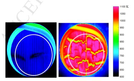
Figure 3: Temperature field in Kelvin and studied area (white circle) at 120 s for two different external heat fluxes ( $20 \text{ kW.m}^{-2}$  (left) and  $55 \text{ kW.m}^{-2}$  (right)).
