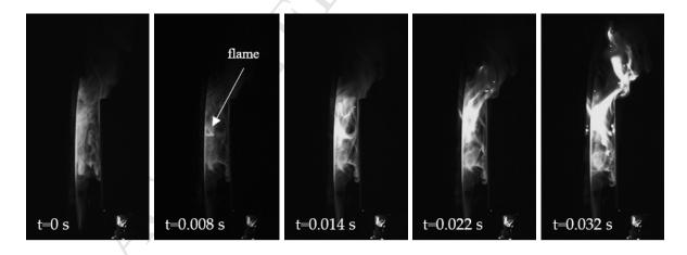
Figure 7: Ignition piloted by cone coil at 75 kW.m<sup>-2</sup>.
