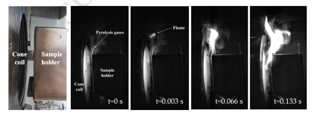
Figure 2: Auto-ignition far from the exposed surface (flaming ignition) at 75 kW.m<sup>-2</sup>.
