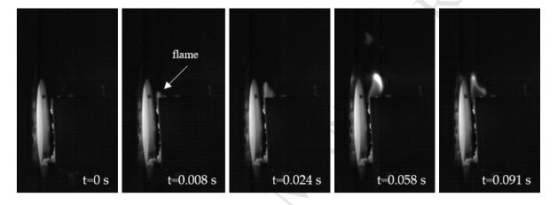
Figure 6: Auto-ignition close from the exposed surface (glowing ignition) at 55 kW.m<sup>-2</sup>.
