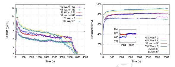
Figure 9: MLRPUA and surface temperature for tests with sample ignition (45 to 85 kW.m<sup>-2</sup>).
