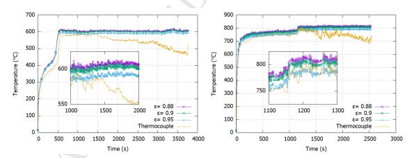
Figure 4: Time evolution of the surface temperature for two different external heat fluxes (20 kW.m<sup>-2</sup> (left) and 55 kW.m<sup>-2</sup> (right)) calculated with the infrared camera for 3 values of emissivity and measured with a thermocouple located at the surface center.
