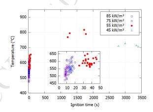
Figure 8: Surface temperature at ignition versus time-to-ignition.
