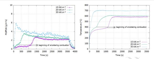
Figure 10: MLRPUA and surface temperature for tests without sample ignition (15, 20 and 35  $kW.m^{-2}$ ).
