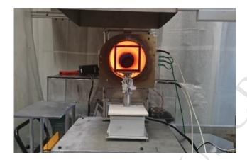
Figure 1: Experimental setup (In this photograph the sample was not put in the sample holder in order to see the cone aperture. The infrared camera looks to the sample through this aperture).
