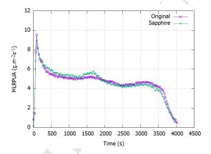
Figure 5: MLRPUA for tests with performed at 55 kW.m<sup>-2</sup> in different configuration.
