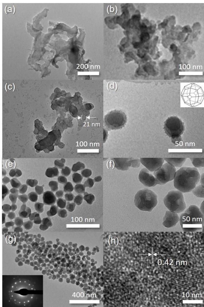
**Figure 4.** TEM images of samples after (a) 15 min, (b) 25 min, (c) 30 min, (d, e) 60 min and (f, g, h) 120 min. Inset of (d) is the theoretical shape of ANA crystalline solid while inset of (g) is the SAED pattern of sample heated for 120 min.
