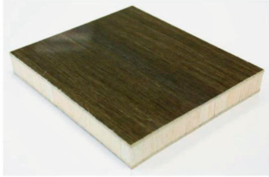
Figure 1. Flax/Elium/Balsa sandwich panel.
