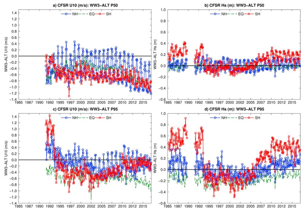
**Figure 1.** Monthly residuals: difference between CFSR reanalysis and altimeter wind speeds (a and c); difference between wave hindcast using CFSR versus altimeter significant wave heights (b and d). Panels (a) and (b) represent the median (P50), and panels (c) and (d) are the 95th percentile (P95). Latitudinal bands are denoted as Northern Hemisphere (NH: 30–60°N), equatorial region (EQ: 30°S to 30°N), and the Southern Hemisphere (SH: 30–60°S). CFSR = Climate Forecast System Reanalysis.
