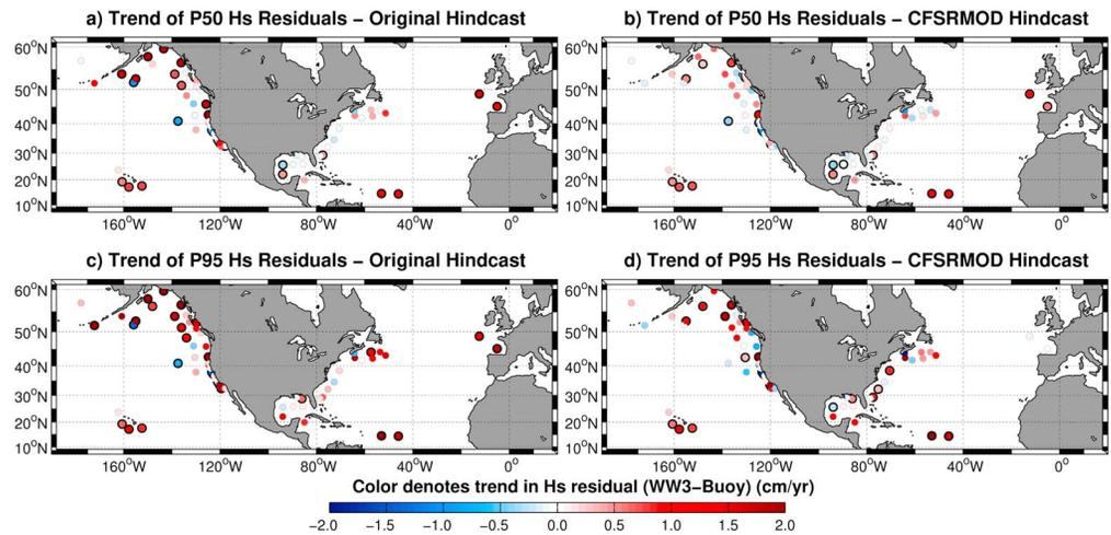
**Figure 11.** Sen's slope computed on monthly  $H_s$  residuals for P50 (a, b) and P95 (c, d) for the original CFSR-forced hindcast and after the hindcast forced by CFSR wind speeds after they were modified (CFSRMOD). Statistical significance at the 95th percentile are denoted by the dark black circle. CFSR = Climate Forecast System Reanalysis.
