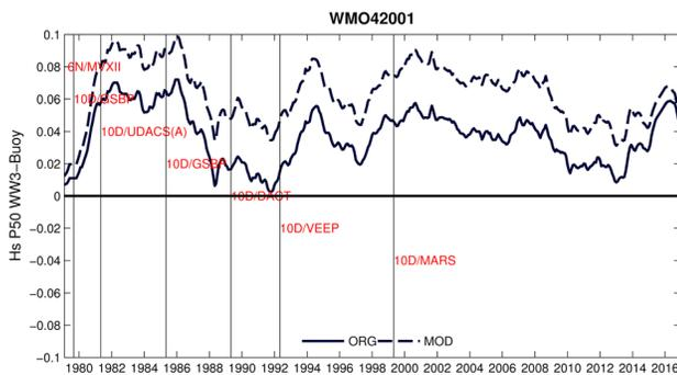
**Figure 13.** Monthly  $H_s$  residuals for P50 at buoy 42001 located in the Gulf of Mexico using the hindcasts before (original: *ORG*) and after modification (modified: *MOD*). The vertical lines and red text denote the buoy hull type and wave sensor payload.
