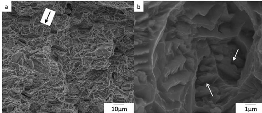
**Fig. 3 – Fracture surface of H-charged D samples tested at 300 °C: (a) macroscopic view, (b) magnification of the area marked by the black arrow – white arrows point to  $\delta$  precipitates.**
