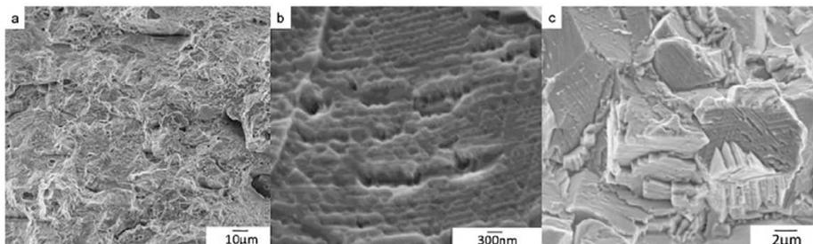
**Fig. 4 – Fracture surface for H-charged C samples tested at 300 °C at (a)  $1.10^{-5} \text{ s}^{-1}$ , (b)  $5.10^{-2} \text{ s}^{-1}$  and (c) tested at 80 °C after a heat-treatment at 300 °C for 30 min.**
