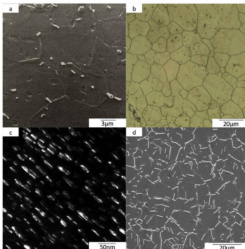
Fig. 1 – Microstructural observations of: (a) Metallurgical state A - SEM, (b) Metallurgical state B - Optical Microscope, (c) Metallurgical state C - TEM, (d) Metallurgical state D – SEM.
