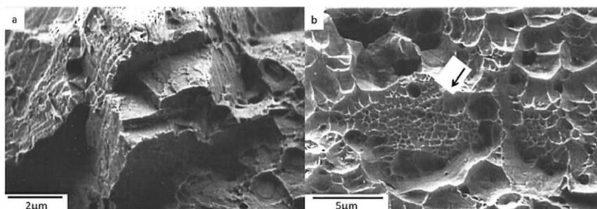
**Fig. 2 – Fracture surface of samples exposed and tested in LWR environment at (a) 80 °C, (b) 300 °C.**
