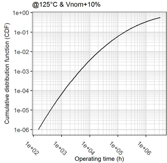
Fig. 6. Failure probability versus operating time for devices at  $125^\circ\text{C}$  and  $V_{nom}+10\%$ .
