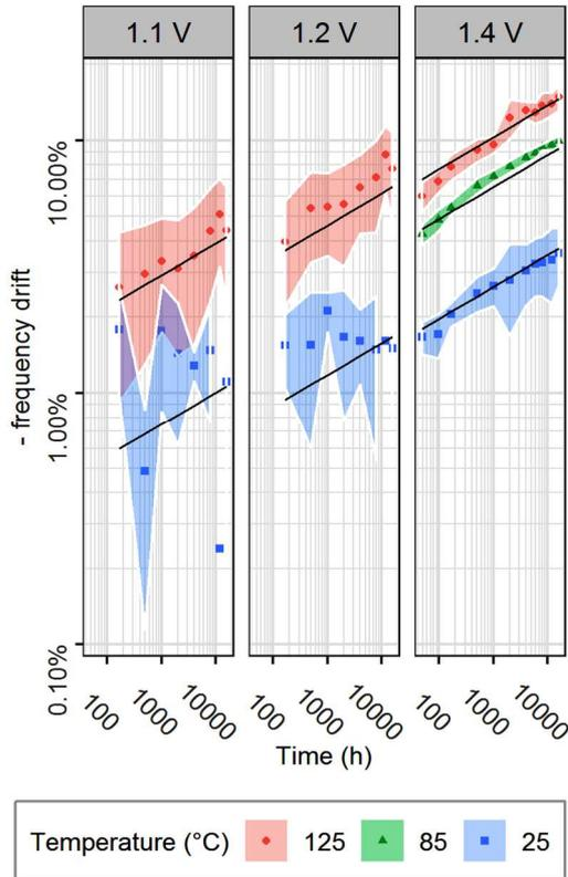
Fig. 2. Evolution of the mean percentage of frequency drifts for each stress condition. Error envelopes are the empirical unbiased standard deviation. And solid black line is the fitted model.
