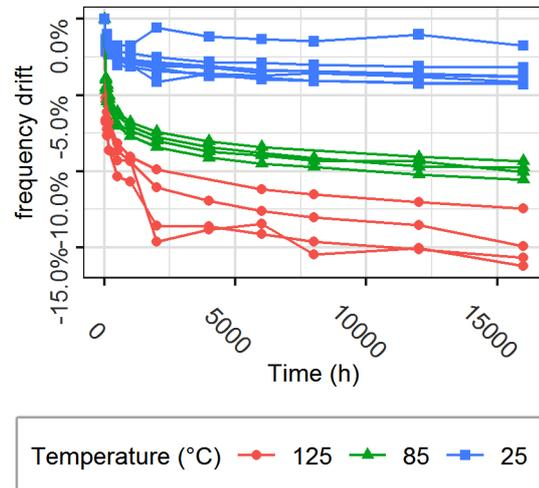
Fig. 1. Frequency drift of DUT aged at 1.4V
