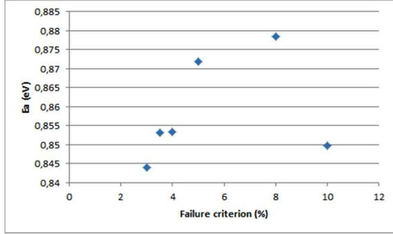
Fig. 4. Evolution of the apparent energy of activation with several failure criteria
