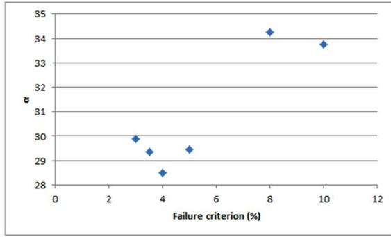
Fig. 5. Evolution of alpha exponent in power electrical acceleration factor with several failure criteria
